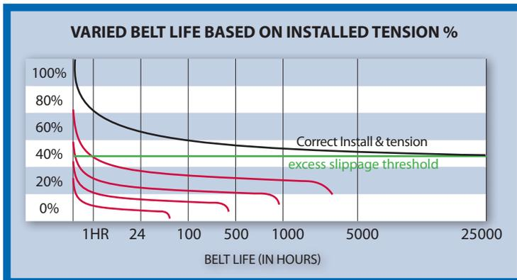
Belt life varies greatly depending on not only how the belt is installed, but on how the belt is tensioned at installation.
