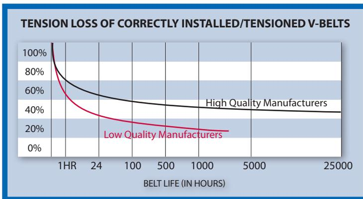
Tension loss occurs on all manufacturer's belts. The highest quality belts still lose nearly 50% of installed tension, while lower quality belts lose over 70% of installed tension. **You cannot "feel" the correct tension on a V-Belt.** On a test given to over 200 experienced maintenance personnel, only 1% tensioned a belt correctly using the "feel" method. Most were at 7%- 50% of correct tension.
