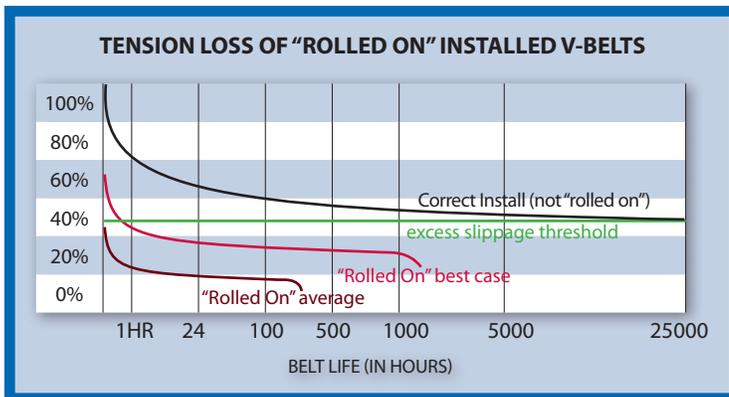
Rolling or prying a belt on a drive gives one of two results, both lead to shortened belt life. Rolling causes low belt tension resulting in low belt life due to slip and heat build up. Prying a belt damages cables in the belt, leading to early belt failure.
