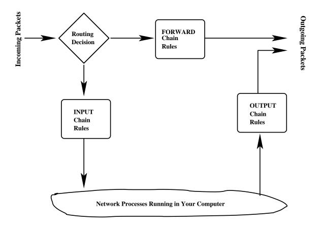
Figure 1: This figure depicts how a packet is subject to the routing rules in the INPUT, OUTPUT, and the FOR-WARDS chains of the filter table. (This figure is from Lecture 18 of "Lecture
